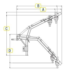
The safest most powerful planetary auger drive attachment range for tractors on the market today. The hydraulic ram provides maximum down pressure for the auger utilizing the full weight of the machine.
